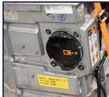
Make sure orange plug is removed and area is protected from contact.
