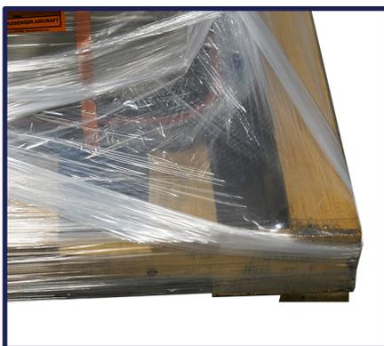
Shrinkwrap to pallet, with wrap extending down around pallet as well as the battery. Make sure enough wrap is used to prevent easy tearing of wrap.
