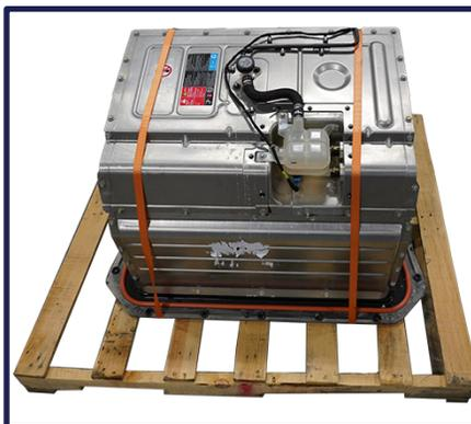
Secure to pallet with vinyl banding over topmost insulating layer.
